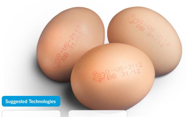
**Continuous Ink** Jet (CIJ) is an ideal technology for in-line coding directly on eggs. It is the costeffective solution because it requires the fewest printers, and the most efficient as printers are integrated with the grader for direct controlling from the console. CIJs also utilize food-grade ink specially formulated to safely adhere to egg shells.
